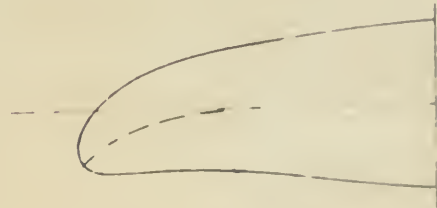
LEADING EDGE NO. 7 ORIGINAL CONTOUR MODIFIED APP. TO 420-- SERIES AIRFOIL REF. DWG. W.T. 179-196 7 OF 7
